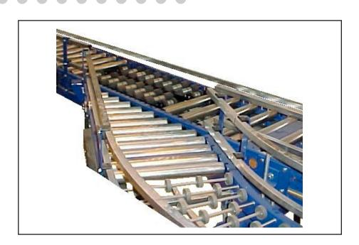
Gravity spurs are used where a secondary conveyor or pick lane needs to feed loads into a main conveyor. The angle of the merge is 30 or 45 degrees and can be bolted to a conveyor straight anywhere along its length.
