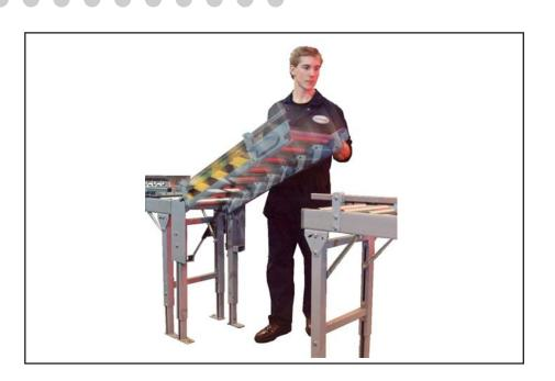
The Gravity personnel gate is designed to allow personnel access through a run of conveyor. It attaches to a conveyor straight and forms part of a straight run of conveyor. It gives 850mm of clear entry and fits into a 1m gap in the conveyor. The gate is lifted manually and gas springs are fitted to reduce the amount of physical effort required.
