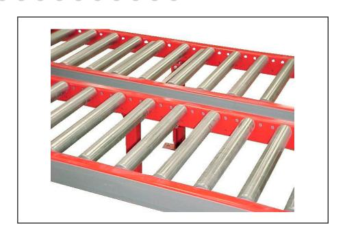
Gravity conveyors are the cost effective solution to many materials handling needs. The rollers reduce surface friction and allow goods to be moved manually without the aid of power. They suit flat based goods or those which are transported in flat based containers, and can support loads up to 110kg per metre.
